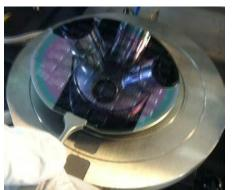
Switch the wafer vacuum ON. By default only the center hole is used but vacuum rings can be activated if necessary by replacing the axial screw in the chuck.
