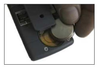
• replace (clockwise) the battery cover back on using the key.
