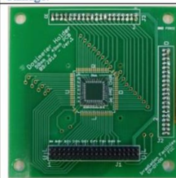
Halogen Free DS-7402, at same levels of radiations doesn't show any considerable damage.
